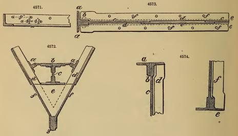
Bulkheads.—See that the bulkhead-frames are all chipped fair on edges, prior to putting up in place, so that the bulkhead plates can be properly calked under the shelf-plates, stringers, and so on.
